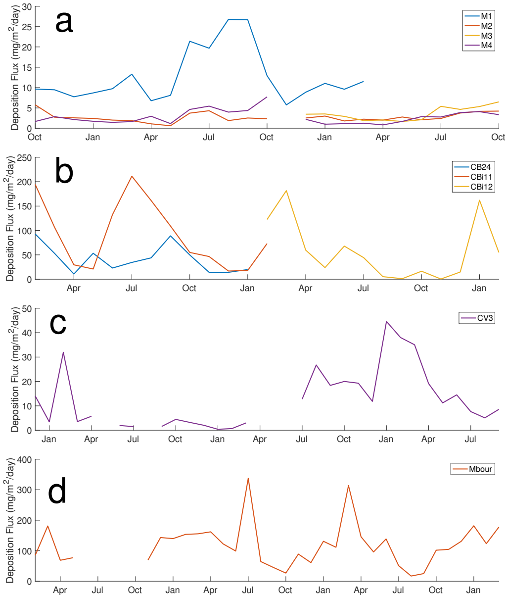
Figure 2.3: Time series of monthly-averaged deposition for all sites, separated by publication source: (a) van der Does et al. (2020) spans October 2012 - October 2014, (b) Friese et al. (2017) spans February 2013 - February 2015, (c) Romero et al. (2016) spans December 2009 - September 2012, and (d) Skonieczny et al. (2013) spans February 2006 - March 2009. The x-axis is marked according to the central month in each season (i.e. January for winter, April for spring, etc.). Deposition for sites in (a) primarily peaked in summer, and there is a pronounced deposition flux drop-off for sites west of M1. Sites in (b) have mixed seasonalities, with peaks in summer, winter, and early spring. Site CV3 (c) had winter and early spring peaks. The Mbour site (d) had peak deposition around summer and spring.
