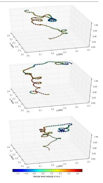
**Fig. 9** Examples of 3D trajectories of the three UAVs from t = 0 s to t = 150 s in the 'No information' scenario. The vertical wind component ground truth is shown in colors. All UAVs start on the bottom at altitude 0.8 km at the beginning of the simulation.
