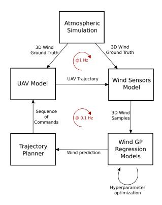
Fig. 8 Simulation architecture.
