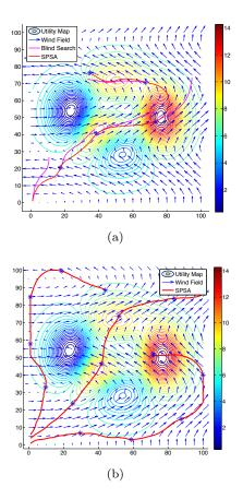
Fig. 5 a) one UAV is moving in a 2D environment where a scalar utility map and a wind field are defined. The trajectories initialized by a blind search at every planning-horizon  $\Delta T$  are shown in magenta, and the final trajectories provided by the SPSA algorithm are in red. b) 3 UAVs are steered in the same environment to maximize the total utility (only the final trajectories are shown).
