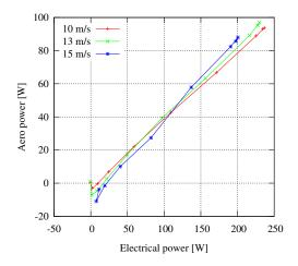
Fig. 21 Resultant propeller aerodynamic power from battery input power for three different flight speeds.
